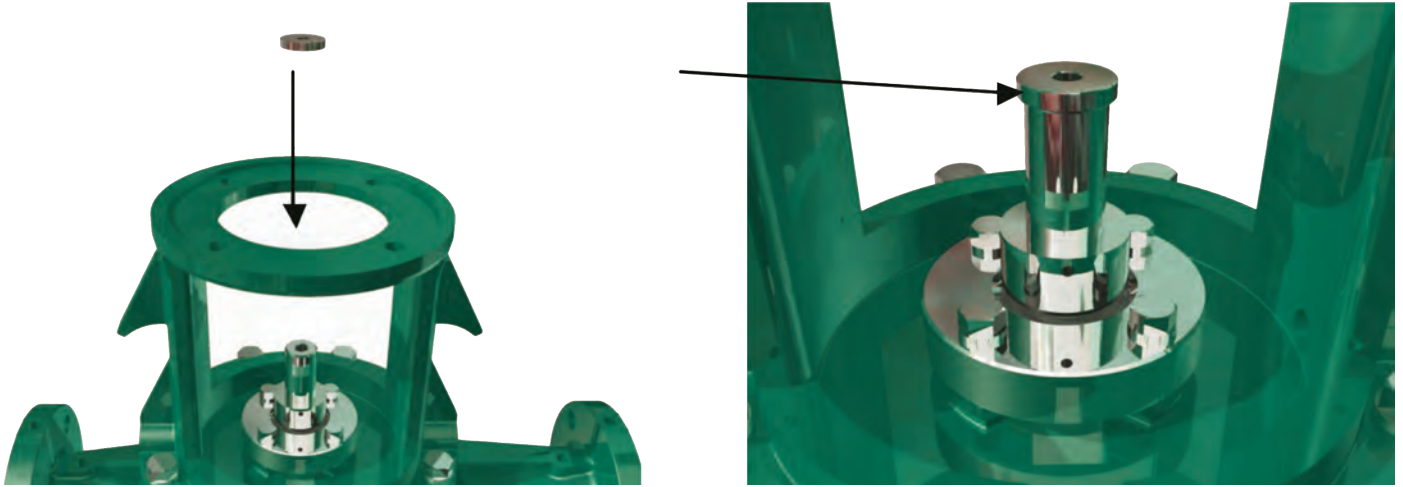
Figure 6.19 Placing the lockwasher on the shaft.
