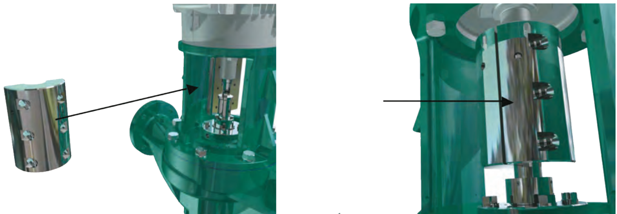
Figure 6.26 Placing the second half of the coupling in the shaft.
