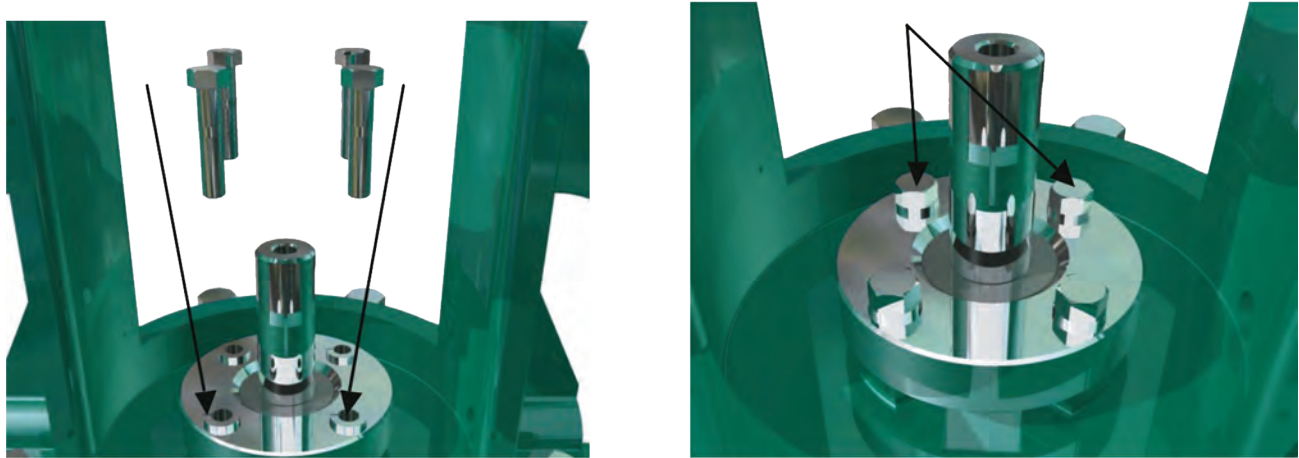
Figure 6.17 Fastening the corresponding screws on the seal gland.
