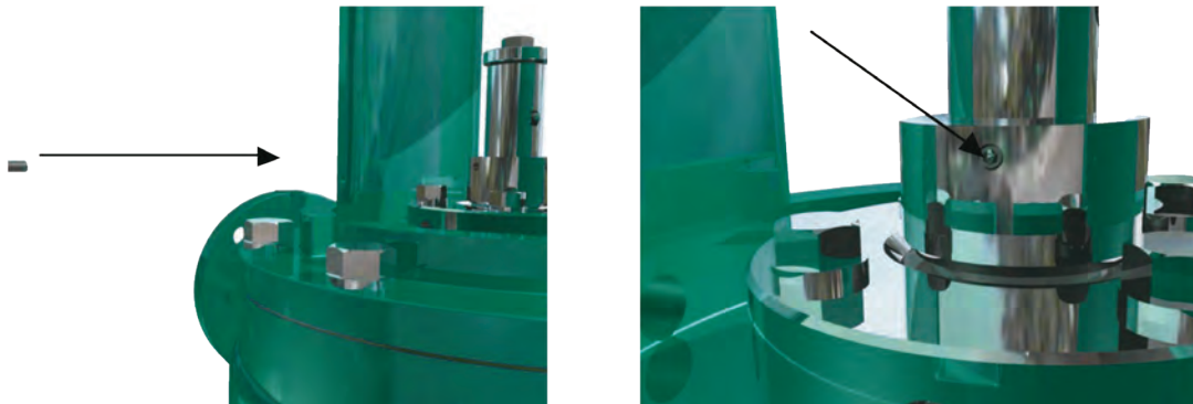
Figure 6.29 Tightening the setscrews of the rotating part of the mechanical seal.
