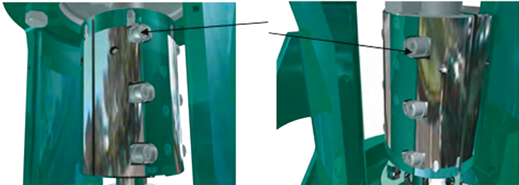
Figure 6.28 Placing and tightening the coupling screws.
