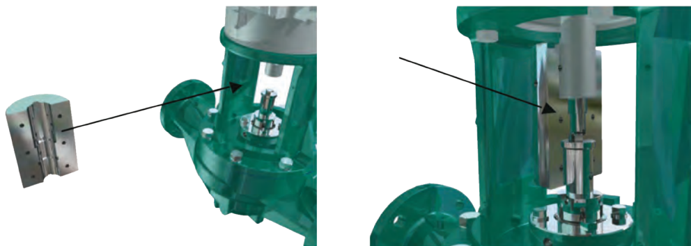
Figure 6.25 Inserting one-half of the coupling and adjust it to the motor and impeller shafts.
